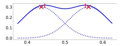
FIGURE 3.2. The red crosses show the true location of  $t_1 = 0.44, t_2 = 0.56$  of two one-dimensional Gaussians, each depicted as a dotted line. The red bars however, show the local maxima of the sum of these gaussians and this sum is shown in a continuous line.
